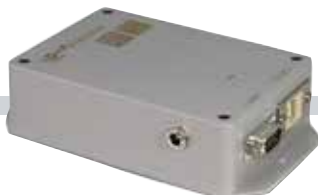
Integrates Somfy RTS and Somfy Digital Network™ (SDN) motorized applications with RadioRA® 2, Homeworks® QS, GRAFIF Eye® QS, and Quantum® control systems.
